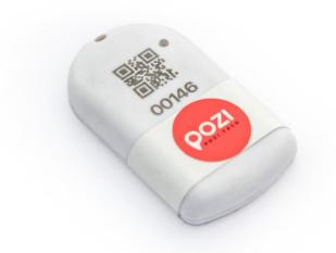
The SafeTag is a handheld device providing UWB-based real-time distance measurements and distance-based safety warnings for pedestrians in the proximity of MHEs equipped with SafeRadar units. The SafeTags have built-in batteries, which can be wirelessly recharged with the SafeTag Charger devices provided.
