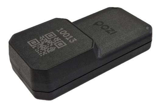
The SmarTag GNSS unit also includes dedicated components to provide remotely controlled visual (LED) feedback functions, as well as a motion sensor to monitor the movement and impact of the person using the device. The SmarTag GNSS EX can be integrated optionally with handheld and portable devices (e.g., smartphones, smartwatches) or other compatible devices using the built-in Bluetooth® Low Energy (BLE) interface.
